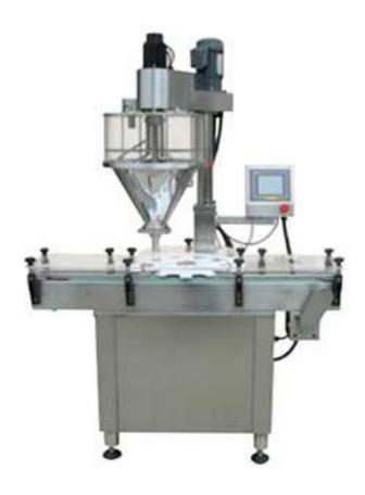
The Model machine could do work of measuring, bottle holding and filling, etc, it can constitute the whole set can filling work line with other related machines, and suitable for filling kohl, glitter powder, pepper, cayenne pepper, milk powder, ice flour, albumen powder, soy milk powder, coffee powder, additive, essence and spice, etc.
