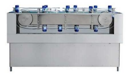
This washer is designed for the three pieces canned food production line. It is small size, high efficiency and automatic. Empty tinplate cans enter into turnover device, then water spray the inner wall of the can to clean the empty cans, after that the water flow into recycle pipe to discharge, and the cans enter into the production line.
