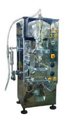
Model AP-Collar- 400P Single Lane pouch filling machines are offered to the clients in various web control options that includes pneumo hydraulic web edge controller and electronic web edge control. The range of machines is widely demanded in the industries for the pouch filling of non free flow powder, free flow powder and granules products.
