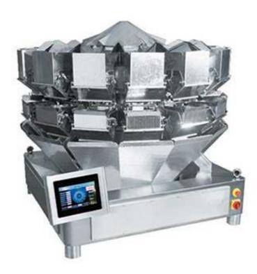
Applicable for weighing of light or bulky products, such as large-sized nuts, vegetables, salads, etc.
