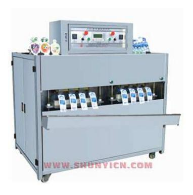
This machine work automatically from filling, pressing bag, sealing and discharge bag, except putting bag manually. Filling full, easy operation and sealing tight.
