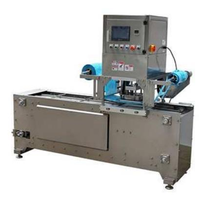
Automatic tray sealing machine can detect filled trays, auto vacuum & nitrogen flushing into tray (optional), auto sealing trays by plastic film, film pulling and positioning, auto printing the produce date(optional), auto collect the waste film, auto discharging the finish products. Base on different mold quantity, its capacity from 800-2400cups per hour, suitable for factory production needs.
