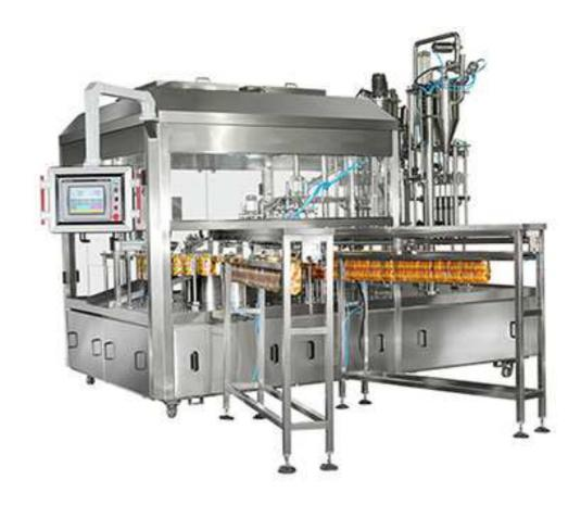
This machine is suitable for filling and capping spout pouch with liquid such as jelly, soy milk, milk, yogurt, pure water, fruit juice, ice cream, edible oil, seasoning, washing liquid, etc.
