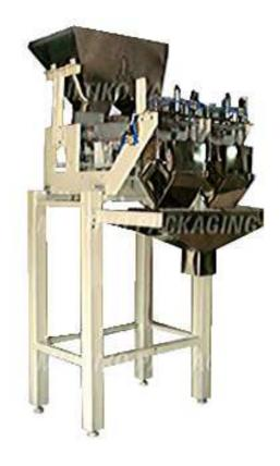
Semi-Automatic linear Weigh scale filling Machine is a very simple machine with Accurate weighing scale equipped with Vibratory feeding system suitable to pack all type products like whole foods, Snacks and various Granules like Sugar, Salt, Tea, Dry fruits, Food Grains, Peanuts etc. in pouches or container.
