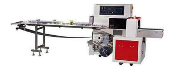
The machine is ideal for packaging solid products with regular shape such as biscuit, bread, candy, commodities and industrial parts. The bulk products need to be placed in a tray to form regular shape first before being packaged
