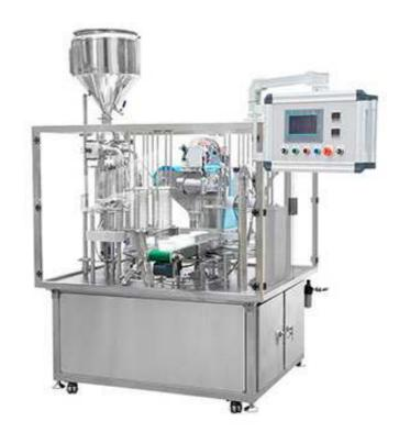
YRC-3 is a filler/sealer produced and designed for medium/large productions. It is perfect for high precision packaging, sealing and checking up to 3600 pieces per hour.
