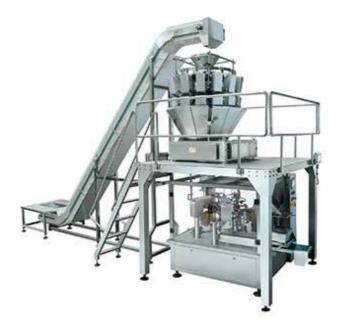
This line mainly installs rotary packing machine, combination weigher and Z-Conveyor, suitable for packing all kinds of grains and solids, such as candy, nuts, raisins, peanuts, melon seeds, potato chips, chocolate, biscuits and so on.
