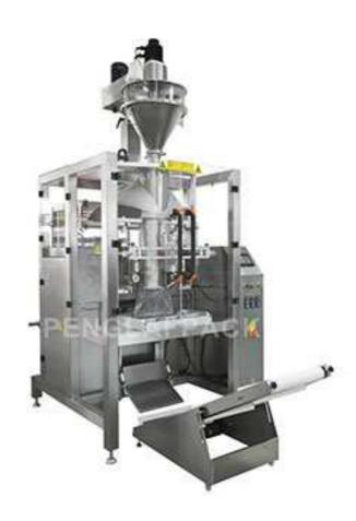
Automatic completion of measuring, bag making, filling, sealing, cutting and printing codes.
