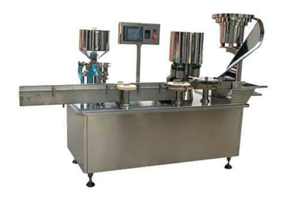
This cream filling and sealing machine is specially designed for cub lose bottles and other largemouth bottles, and it can automatically finish the work of bottle feeding, filling, capping, and sealing. Its rotary valve structure is quite suitable for filling cream and liquids with small particles.
