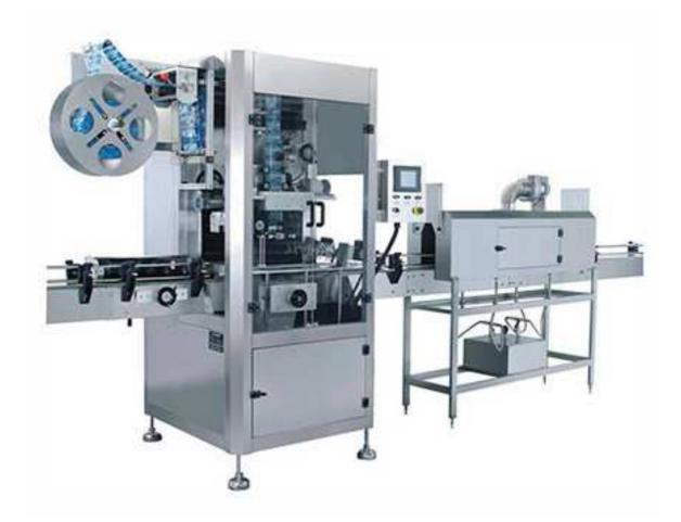
The Automatic Single Head Sleeve Shrinking Labeling Machine adopts international advanced technology, cover the circle label on PET bottle / glass bottle, then heat shrinking to fix on the position which bottle body designated. It is controlled by micro-computer and automatic detection. It is suitable for both PET bottle and glass bottle, The sleeve shrink label material can be PVC or PET material.
