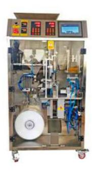
The FF-T10 floor type tea vacuum packaging machine is suitable for various small products vacuum packing such as tea, nuts, preserved fruit, small electrical components etc. The tea vacuum packaging machine whole process is automatically controlled by the vacuum machine. Extraction, sealing, cooling time is adjustable, with digital display every movement of the time, easy to operate. Packing about 10 seconds one time.
