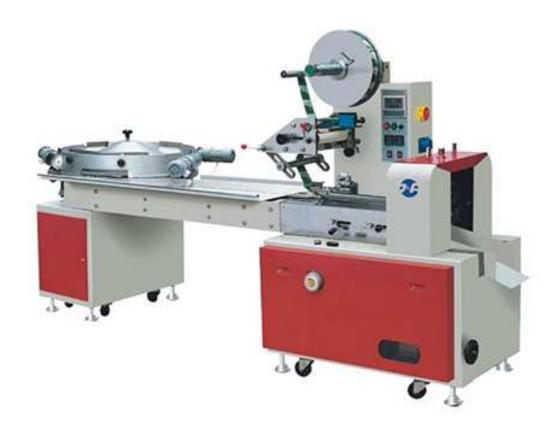
Full-automatic packager is applicable for packing oblong, quadrate, round, oval and shaped candies. With rapid computer programming and photoelectric tracing, Frequency control for stable and free running, Reversible outsize candy sorting disc enables empty package rate to get optimal effect; Excellent performance, simple operation and high-speed package of the whole machine.
