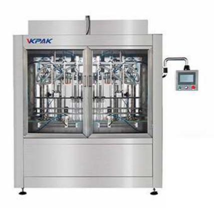
This Automatic Piston Type Sauce Filling Machine is piston type filling machine special made for filling cream or liquid foodstuff such as ketchup, sauce, honey, jam, peanut butter, mayonnaise, salad dressing etc.
