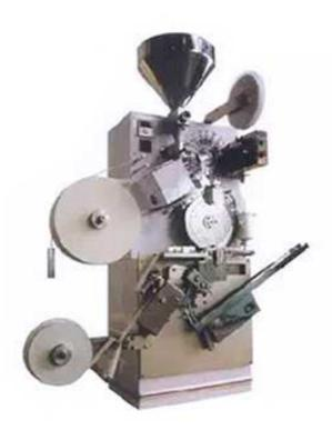
The Tea-bag Packing Machine model CCFD6 have general functions such as automatic ration filling, heat-sealing of tea bag, automatic plastering cotton thread and tag, envelope is cold-sealed by tow-side in longitudinal direction.
