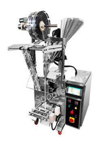
The automatic milk powder packaging machine can pack a variety of powders, and the packaging speed is 30-80 bags per minute, which greatly saves labor costs.
