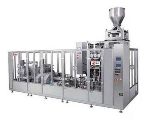
Automatic vacuum packing machine can be used the manipulator to automatically take the bag, and open, automatically print the production date and batch number, automatic feeding and vacuum packaging, completely realize the unmanned operation, and truly realize the automatic packaging.
