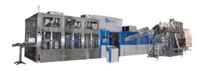
XLOGX24A Description: Spring cramps are used in the bottle washing process; the empty bottles can be turned over180° along the conveying rail. There are two times of internal and external washing, the efficiency of bottle washing is high. The magnetic torque is used for screw capping.
