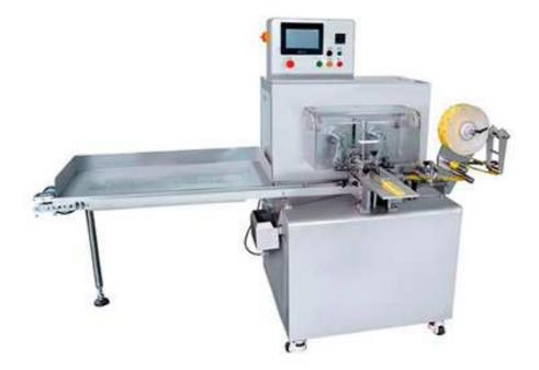
This machine is used to pack solid square and retangle products with flat bottom such as bouillon cube, enveloper-wrapping chocolate, and candy etc.
