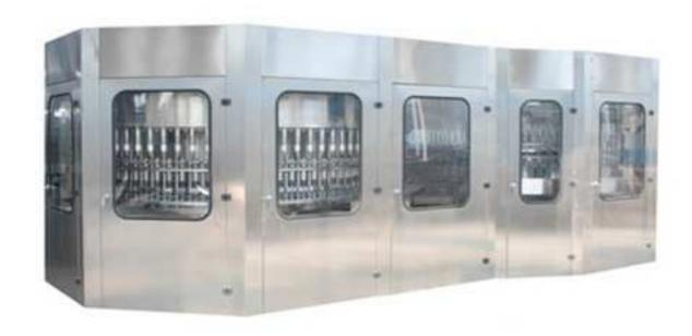
This automatic mineral water filling machine mainly used in the water filling operations, the three function of bottle washing, filling and capping are composed in one body of the machine, the whole process is automatic, it is conveniently trunked to adjust the machine to fill various types of bottles, the filling operation is faster and more stable due to the advanced filling valve technology, The famous brand programed controller (PLC) is adopted to control the machine runs automatically.
