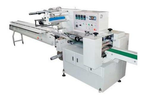
It consists of main machine, input conveyor and output conveyor. The main box is welded with thick 12mm steel plate and made by special heat treatment. The packaging machine and food contact parts are all SU304 food sanitary grade stainless steel materials.
