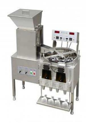
YL-4 is a new design for laboratory production and small batch capacity manufactured. Desktop style for tablet & capsule count but small size and light weight. Once start with one bottle and automatically to count the next when finished, easy picking up and putting down the bottle by hand.
