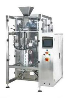
Vertical automatic bag sealing packaging machine is suitable for various snacks, potato chips, banana chips, rice popcorn, chocolate chips, rice, grain, granule, seeds, beans, nuts, cashew, nut cracker, dry fruit, sunflower kernels, corn beans, puffed food, crispy rice.
