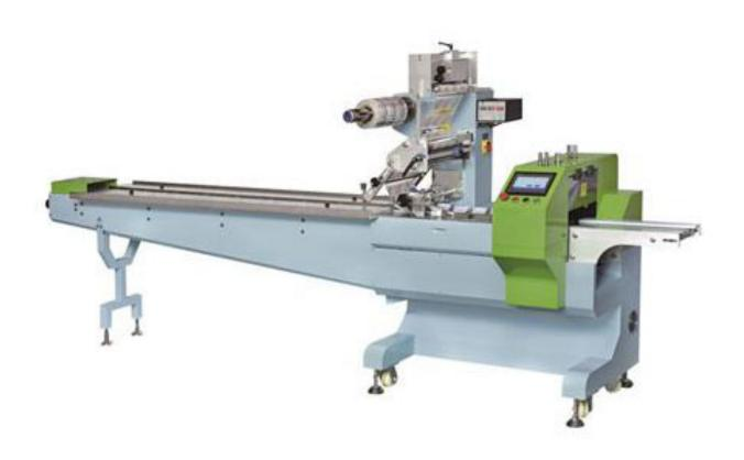
The servo motor in the MK-300S series precisionflow pack wrapper ensures this is a semi-automatic continuous packaging equipment, and is applicable to packaging bread, biscuits, instant noodles and other regular items. This wrapper features an adjustable packaging length according to the items that need to be packaged, and the servo motor ensures an exceptionally high accuracy. The independently controlled PID temperature is also suitable for a large range of packaging materials.
