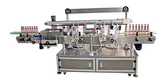
It is especially designed for more big taper bottle products to realize the body & neck double taper labeling.
