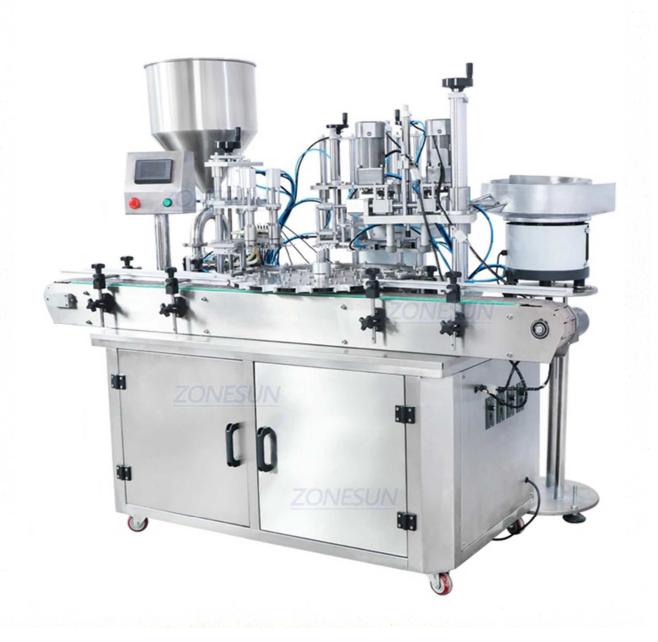
This automatic production line is designed with multiple function, it can arrange bottles, fill liquid or paste, feed bottle plugs and caps, cap bottles and sort finished products automatically. It can help you improve working efficiency. This is suitable for essential oil, water, juice etc. We can customize the machine and make it can work for different sizes of containers at the same time.
