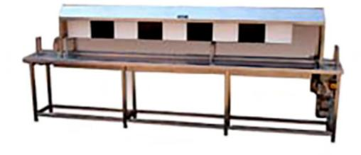
We offer Online Visual Bottle Inspection Machine that is fabricated using S.S square pipes and is supported on adjustable bolts. These are widely used in pharmaceutical processing industries all across the globe and consist of three-track conveyor with stainless steel structure and square pipes with moving S.S. slat chain and supported on adjustable bolts. These are incorporated with hood and lighting arrangement with visual inspection background of alternate black and white color
