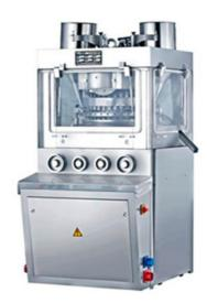
It is mainly used in pharmaceutical industry and also the chemical, food, electronic industries, for pressing various granular raw materials into tablets.
