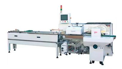
Great packaging solution for soft items, vegetables, and fruits, etc., the wrapper produces finished packages with less air and achieves optimal hermetic sealing. Flow pack machine for frozen cakes, ice pops, cheese, etc.
