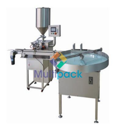
We specialize in deliver custom ointment filling machine that can be used to fill various products like bam, hot balm, molten, wax, lip balm, cream etc in molten condition. We provide machines to fill viscous and semi viscous fluids in various types of containers. The machines are auto piston type that is rational in design, compact with pneumatic components. Our machines are popular providing disturbance free heavy duty performance and available at the most affordable rates.
