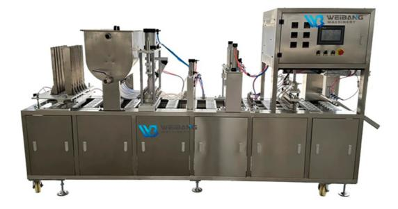
This machine is the mufti-functional and advanced yogurt cup filling machine. It is featured with automatic dispensing cup, twice filling, twice sealing, cover pressing and exit of 2, 4, 6, 8, 10 cups one time. It is suitable to milk, juice, honey, water and granular, powder, fruit, crisp and so on.
