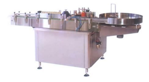
This adhesive label machine pastes automatically. With additional supplying equipment, giving bottles, pasting and sticking labels can complete once. The place of sticking label is in order. After refitting, it can stick 2-3 labels on round bottle at one time. This machine is suitable for the trades of foodstuffs, pharmaceutics and chemical industry for labeling.
