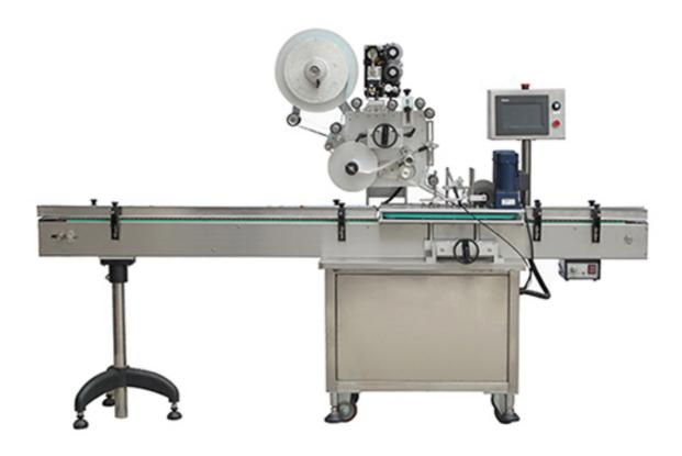
ALT-B is suitable for flat or quadrate containers widely such as cigarettes, bags, cards & toothpaste boxes, etc. The machine is economical and easy to operate, equipped with a friendly HMI and PLC control system. The performance is stable with a level off especially at the top of the container. The system easily changeover based on the requirement.
