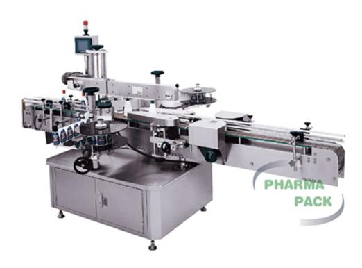
The bottle without label enters the rectifying belt by bottle dis pen sin g wheel, two clamping belt orients bottle, and top belt keeps the bottle's pose. After the object detecting sensor senses bottle, it sends a dispensing label signal to la bel dispenser. At this time, bottle is labeled by label dispensing board. Meanwhile, the base paper is rolled back and label is labeled closely and levelly to bottle by the special device.
