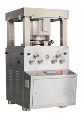
This machine is a double-press type; it continually and automatically tablet press granular raw materials into round tablet, irregular tablet, carved tablet and two layer (color) tablets etc. It is mainly used in pharmaceutical industry and also the chemical, food, electronic industry and so on.
