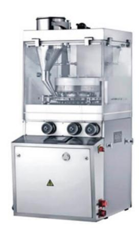
This machine is suitable for pressing various kinds of granular materials into round tablet or different geometrical shape tablets, specially for small-scale batch production.
