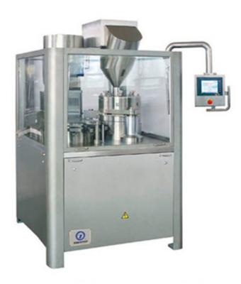
This machine is an intermittent motion and dosing disk type automatic capsule filler, it's widely used for filling medicine powder/granule/pellet in pharmaceutical and nutrition industries etc.
