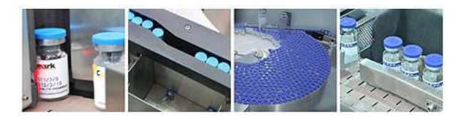
A simple wrap-around labeling system specifically designed for the need of the pharmaceutical industry for labeling on small vials. Optional inspection and rejection devices for missing or wrong code, missing labels to ensure output quality. Capacity up to 350ppm.
