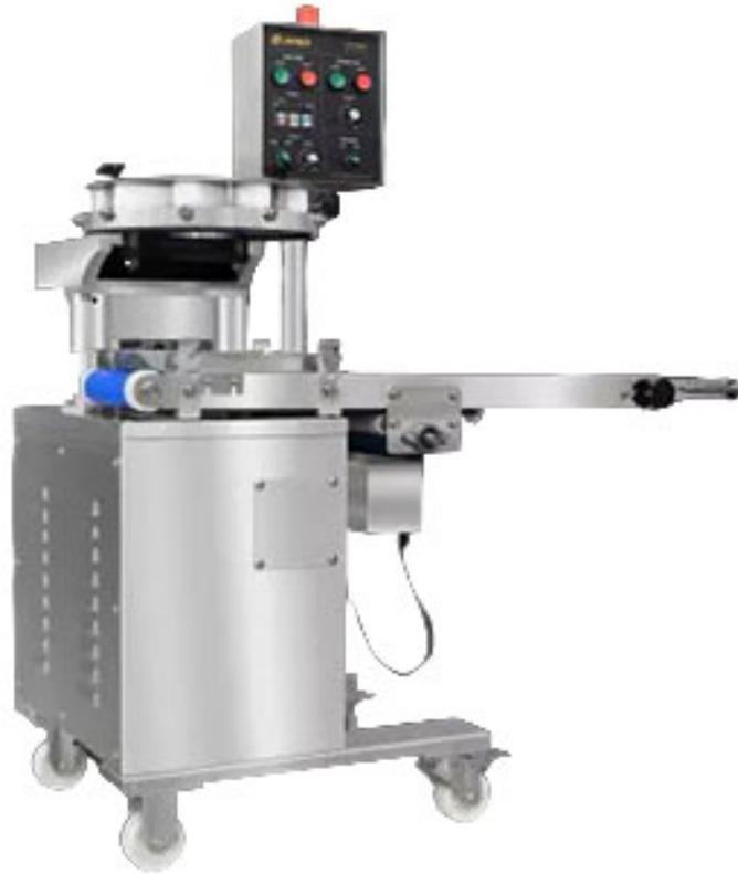
The EA-100KA is a high-efficiency forming machine with an independent motor control system. The Forming Machine can work with HLT Series to produce various products such as mini juicy bun, meat bun, beef roll, baozi and the like with or without pleats. Its maximum capacity is up to 6,000 pieces per hour.
