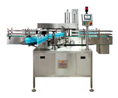
Water Bottle Labelling Machine is suitable for automatic labelling 200 ml to 2000 ml PET bottles with Up to 120 Labels per minute Output Speed. The Machine incorporates the latest sophisticated Micro Processor Control Label Dispensing system with a user-friendly sensing system for labels and products.
