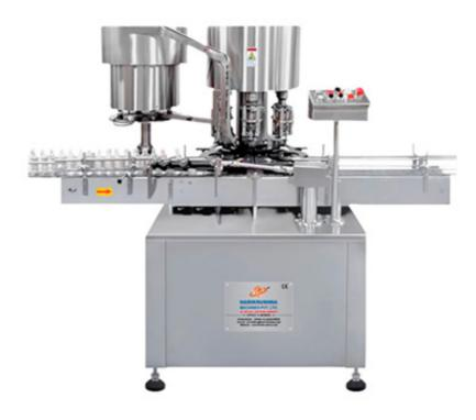
The Automatic Rotary ROPP Cap Sealing Machine consists of a main structure, product transmission belt with an adjustable guide, in-feed screw, star plate, sealing heads, vibratory bowl for caps, cap delivery chute, product's height adjustment screw, safety acrylic cover (OPTIONAL), electrical panel, motor, sensors & AC drive.
