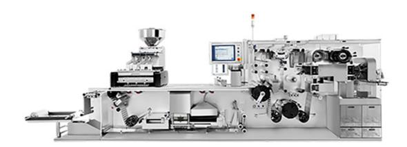
HM 600 is a blister packaging machine in a continuous / intermittent motion with single to three lane mode of operation. This model is suitable for large sized production, in which is capable of producing up to 600 blisters per minute. (900 blisters in 3 lane mode) HM 600 offers gentle and high performance for all types of solid dosage products with common type of forming material. Depending on the product type, either platen or rotary type of sealing method can be applied.
