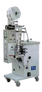
This kind of small and middle size automatic liquid packing machine is typically used for packaging the pure liquids of foods, medicine, and chemicals, such as water, wine, oil, shampoo, liquid pesticides, and the like. And its packaging materials can be various heat-sealable composite packaging materials, like paper, cellophane, BOPP film, tea filter paper, and more.
