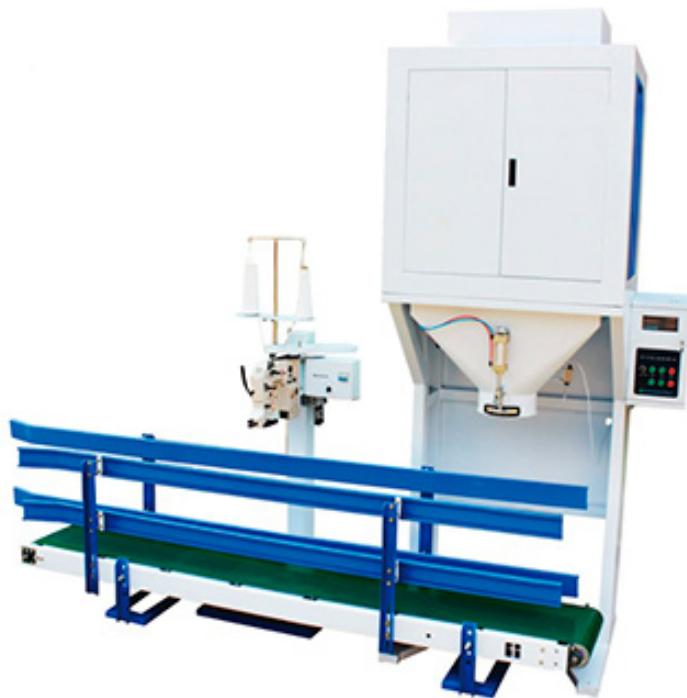
The total unit includes one set of DCS-50 automatic weighing machine, one set 2.5 meters belt conveyor, one set of sewing machine, used for weighing filling granules, such as: rice, seeds, grains, etc. in pp woven bags and sewing the bag.
