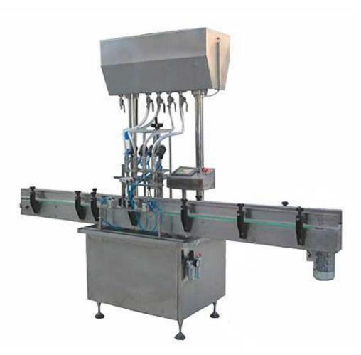
This machine is suitable for filling disinfectant, pesticides, oil, and high-dose beverage. This machine adopts flow-type filling, PLC control, touch screen operation. The filling volume can be adjusted easily.
