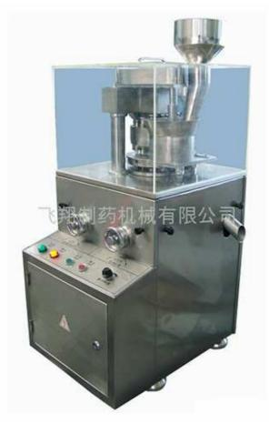
ZP5D Rotary tablet press is a new generation product by our factory, and this machine is a single roller continuous automatic tablet press for pressing various kinds of different shape tablets and plain tablets, such as round tablet, irregular tablet and carved tablet etc.
