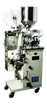
This troche packaging machinery is typically used for packing tablets, buccal tablets, pills and more, and it is widely used in industries of medicine, food, chemical and the like.
